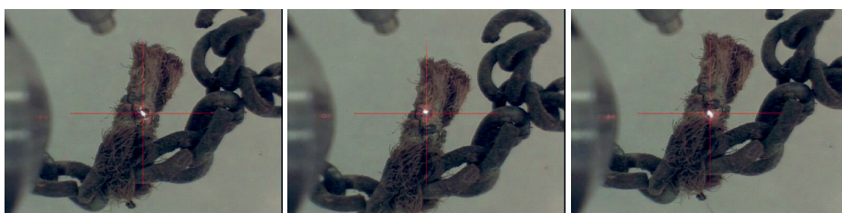
Measuring points (10, 11 and 12) on metal fragments on textile thread
